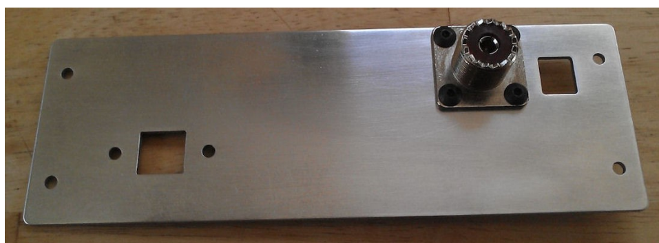
New Rear Panel with SO-239 Connector
